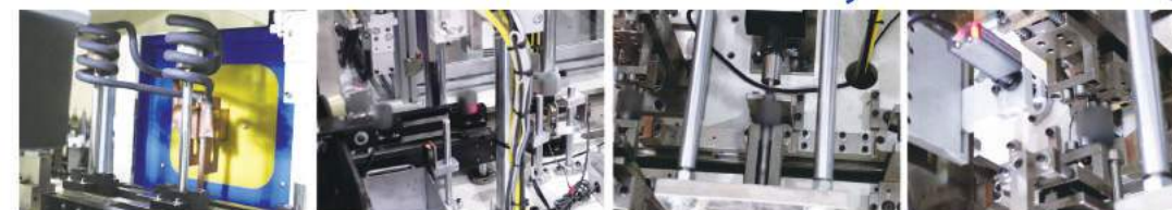
高週波機加熱鐵芯 High frequency heating lamination 矽鋼片厚度檢測 Lamination thickness detection 軸芯脫拔力測試 Shaft pull-off tester 偏擺測試機 Run-out test
