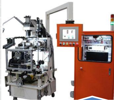
Riveting Joint Equipment
